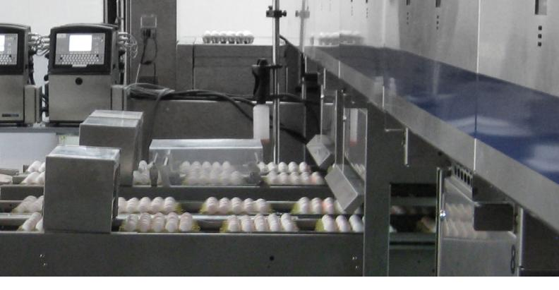
In most cases, printing equipment that is integrated directly with the grading equipment will maximize the results of your significant grader investment. For older existing grading equipment, understand that there may be additional grader investments required. Work closely with the grader manufacturer to understand the integration options. Tight grader integration is beneficial, because the grader will control the printing equipment directly and will ensure the right code is on the right egg.
